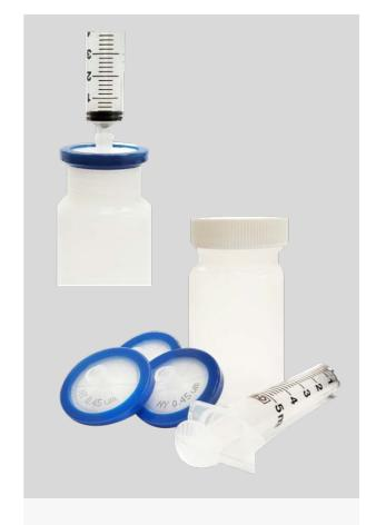
Note: Each new sample location must be filtered using a new syringe and filters to avoid contamination.
